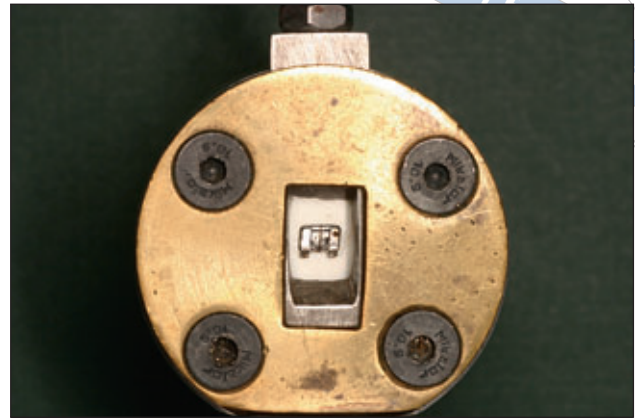
Fig 1 SBS-testing device that avoids the generation of leverage forces.
